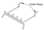
Figure 7 - Attaching Grate Steps
